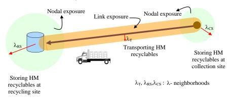
Although in most cases, the HM has a radius of spread (r) proportional to the third root of its quantity (Q), in this research it is assumed that the radius of spread in case of storing facility is a function of the square root of quantity i.e.  $r \cong \sqrt[2]{Q}$ , similarly to the idea deployed by Current and Ratick (1995). This approximation gives opportunity to easily calculate risk  $R_j^F$  imposed by storing facility j as a area of circle of the radii  $\sqrt{Q_j}$ :
